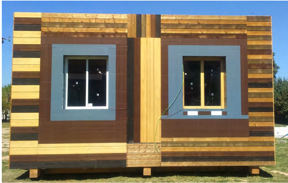
Figure 4. Samples to be tested. On the left side Reference Window, on the right side Optimised Window.
