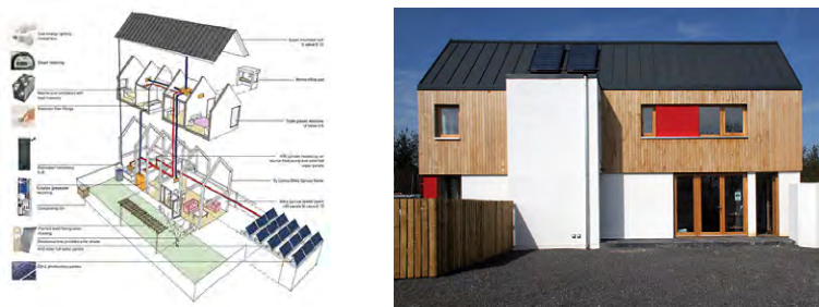
Figures 8&9. Axonometric of Ty Unnos components and environmental strategy; Longhouse south elevation.
