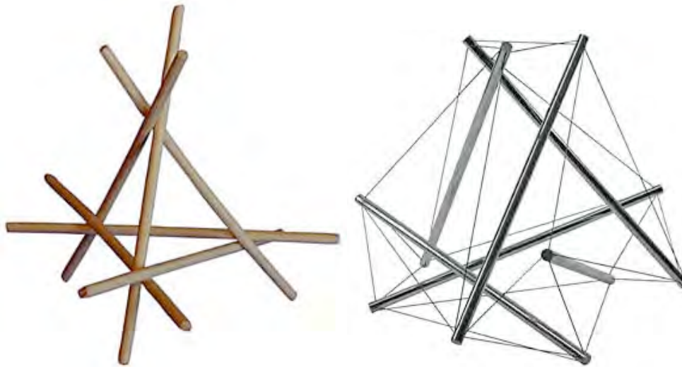
Figure 4 - Helicoidal tetrahedron and its equivalent tensegrity
