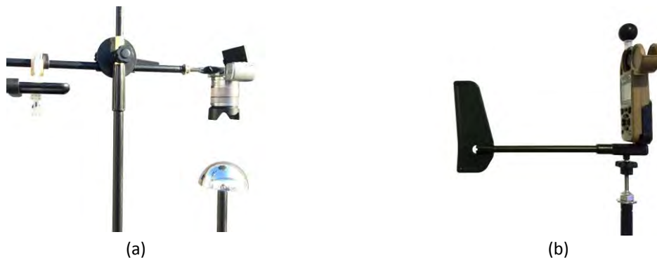
Figure 1. The experimental setup: (a) the hemisphere and DSLR camera, (b) Kestrel 5400 Heat Stress Tracker.
