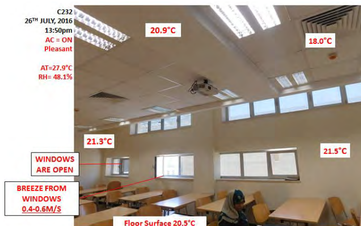
Figure 8. Spot measurements taken in classroom C232.
