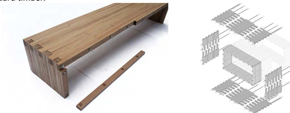
Figures 2&3. Tectonic model of table; and axonometric exploring additive, small section, short length construction
