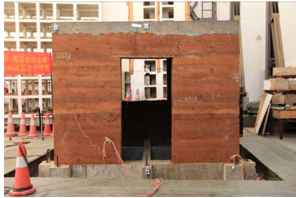
Figure 12. The state of model after test
